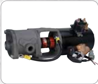
FLUID-LESS PRIMER Positive displacement rotary vane vacuum pump for 20' - 28' suction lifts
